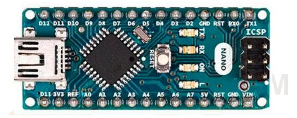
This Arduino Nano is Original Arduino Nano Board. It is a breadboard-friendly board based on the ATmega328P from Arduino officials made in Italy. It has more or less the same functionality of the Arduino Duemilanove, but in a different package. It lacks only a DC power jack and works with a Mini-B USB cable instead of a standard one.
